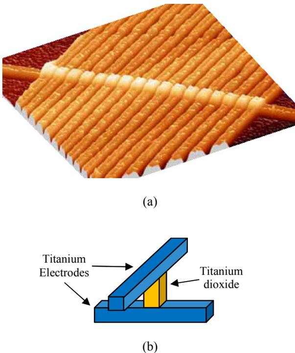
Fig. 3. a) Atomic force microscope image of the  $1 \times 17$  array of  $50 \times 50 \text{ nm}^2$  memristor. b) Schematic illustration of the connections of titanium electrodes with titanium oxide (Williams, 2009).
