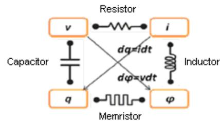
Fig. 2. Four basic passive circuit components (Ho *et al.*, 2009).
