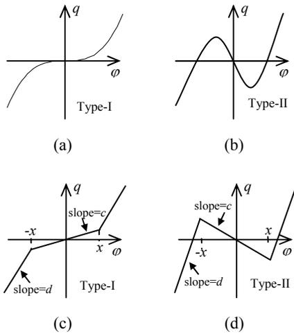
Fig. 3. The terminal characteristics for two types of mductance functions; a,b) the actual c,d) piecewise linearly approximated.
