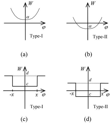
Fig. 4. Mductance characteristics in (7) and (8) for two types; a,b) the actual, c,d) piecewise linearly approximated.
