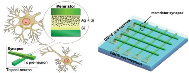
Fig.1. Nanoscale application of the memristor as a synapse. (a) Schematic illustration of the concept of using memristors as synapses between neurons. (b) Schematic of a neuromorphic with CMOS neurons and memristor synapses in a crossbar configuration (Jo *et al.*, 2010).
