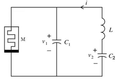
Fig. 6. The 4EC Circuit with a memristor.
