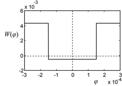
Fig. 7. Piecewise linear memductance characteristic for the 4EC circuit with the memristor.
